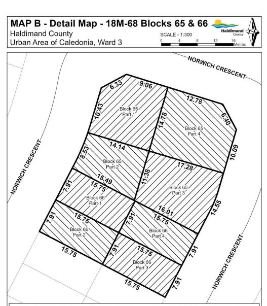
NOTE: Measurements shown on this plan are in metres and may be converted into feet by dividing by 0.3048. Measurements indicated in this drawing are representational in nature. They have been obtained without the benefit of legal or cadastral surveys linked to coordinates and therefore should not be considered to be survey grade and should not be used for legal purposes.
