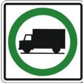
Rb-61 Truck Route Sign
